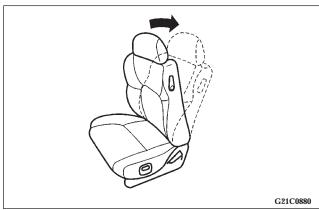
Just by pushing the seatback up into position will lock it in the memorized position.
